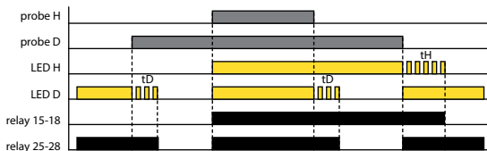
PUMP DOWN, OFF DELAY (Function 6)
