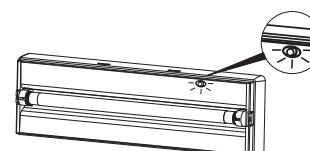
Green LED: mains supply present and battery charge in progress
