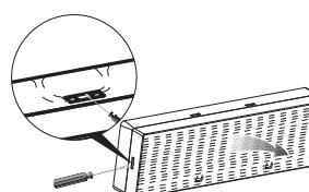
Open the up cover of the luminaire by unlocking the latches for changing the fluorescent lamp.
