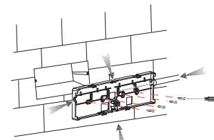
Mount the back cover by screw where you want to fix the luminaire.
