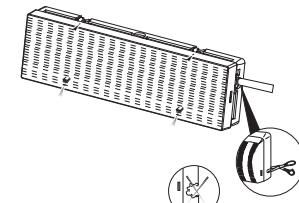
Cut the selected area properly by cissor for luminaire wiring connection.
