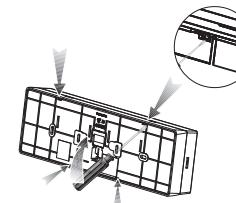
Unlock the side latches by screw driver and pull up the back cover
