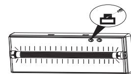
Test Button: After removing the plastic cover, press the button by a screwdriver. The battery sets in and lets the fluorescent lamp.
