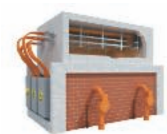
Testing furnace of a materials' testing institute (MPA)
