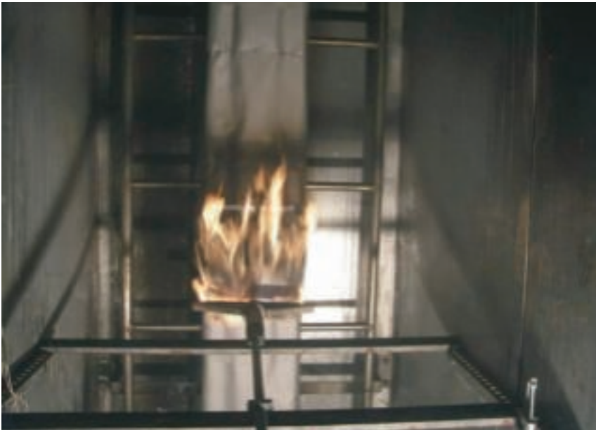
Flaming of the fire protection bandage
