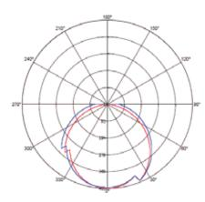
C0 Plane beam angle(50%) FC C00 Plane beam angle(50%)
