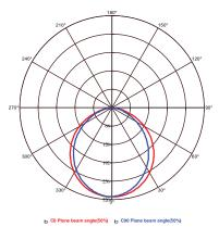
C0 Plane beam angle(50%):109.5(DEG) C90 Plane beam angle(50%):99.1(DEG)
