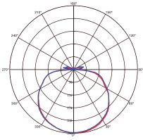
b C0 Plane beam angle(50%) C0 Plane beam angle(50%):137.3(DEG) C90 Plane beam angle(50%):138.8(DEG)
