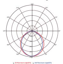
C0 Plane beam angle(50%):109.5(DEG) C90 Plane beam angle(50%):99.1(DEG)
