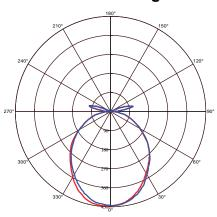
C0 Plane beam angle(50%):102.1(DEG) C90 Plane beam angle(50%):101.4(DEG)
