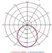
C0 Plane beam angle(50%):105.3(DEG) C90 Plane beam angle(50%):105.5(DEG)
