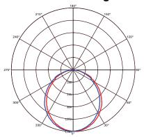
le(50%) b C90 Plane beam angle(50%) C0 Plane beam angle(50%):105.3(DEG) C90 Plane beam angle(50%):105.5(DEG)
