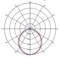
b C0 Plane beam angle(50%) b C30 Plane beam angle(50%) C0 Plane beam angle(50%):105.3(DEG) C90 Plane beam angle(50%):105.5(DEG)
