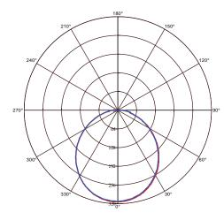
b C0 Plane beam angle(50%) b C90 Plane beam angle(50%) C0 Plane beam angle(50%):107.1(DEG) C90 Plane beam angle(50%):107.0(DEG) Product&Family Code: 071 008 0012
