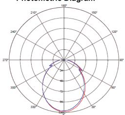
C0 Plane beam angle(50%) C90 Plane beam angle(50%) C0 Plane beam angle(50%):93.4(DEG) C90 Plane beam angle(50%):93.0(DEG)
