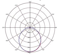
b C0 Plane beam angle(50%) b C90 Plane beam angle(50%) C0 Plane beam angle(50%):107.1(DEG) C90 Plane beam angle(50%):107.0(DEG) Product&Family Code: 071 003 0006
