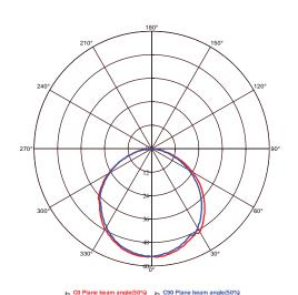
C0 Plane beam angle(50%):112.6(DEG) C90 Plane beam angle(50%):109.9(DEG)
