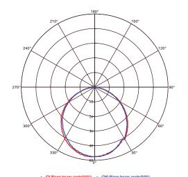
C0 Plane beam angle(50%):111.0(DEG) C90 Plane beam angle(50%):108.3(DEG)
