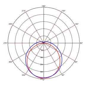
C0 Plane beam angle(50%) C90 Plane beam angle(50%) C0 Plane beam angle(50%):110.3(DEG) C90 Plane beam angle(50%):127.5(DEG)
