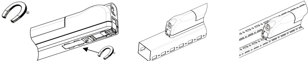
Magnet and screwing - hole centre distance from 455 to 475 mm
