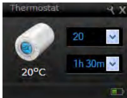
Figure 4.28: Danfoss Thermostat - Parameters Modification Window
