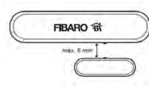
Figure 4.12: Door Window Sensor - correct positioning of the sensor and the magnet
