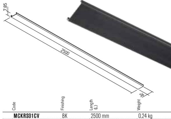
Front cover for masking the remaining open areas in the recessed or surface profiles after installing the light fittings.
