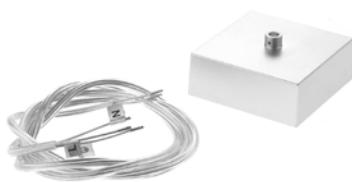
**PRF080PK MWH** Ceiling cup of polycarbonate, for electrical connections masking. Steel fixing clamp, 2P+N (10A/250V/2,5 mm<sup>2</sup>) block of terminals, power supply cable 3x1,5 mm<sup>2</sup>, transparent silicone coating, with a length of 1,5m.
