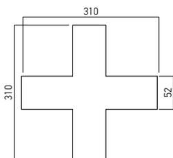
**PRF080XC01** Structural element of aluminum, for cross connecting of four profiles PRF080. Equipped with satin polycarbonate diffusers.
