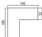
**PRF080LC01** Structural element of aluminum, for connecting at 90° of two profiles PRF080. Equipped with satin polycarbonate diffusers.
