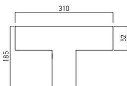
**PRF080TC01** Structural element of aluminum, for connecting in T of three profiles PRF080. Equipped with satin polycarbonate diffusers.
