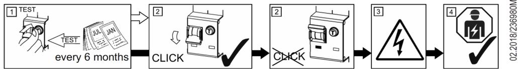
Switchgear must be tested by **PUSHING the TEST BUTTON** every six months. The switch must release immediately. The examination is the responsibility of the user! BS7671:2001, Requirements for Electrical Installations.
