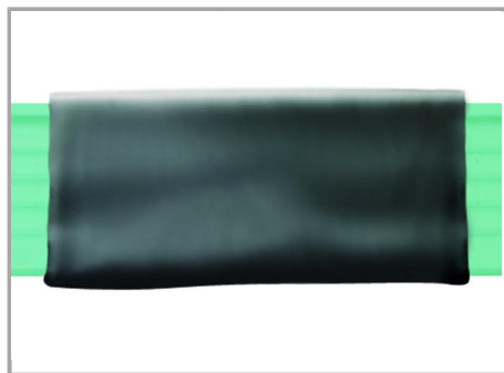
After removing the module, the contact holes in the flat cable must be sealed using insulating tape.
