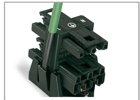
To release the distribution connector, unlock the latch using a screwdriver.
