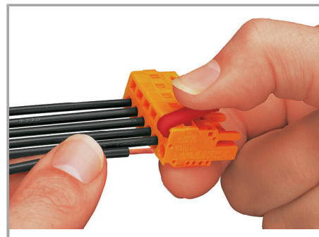
Inserting a conductor into CAGE CLAMP® unit via operating lever (231-291).
