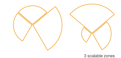
sensIQ detection zone Mounting height 1.8 m black = tangential walking direction orange = radial walking direction
