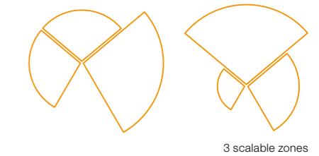
sensIQ S KNX detection zone Installation height 1.8 m black = tangential walking direction orange = radial walking direction
