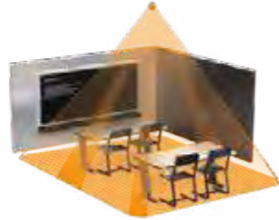
Classroom situation, detection by the Presence Control Pro IR Quattro with square detection characteristic
