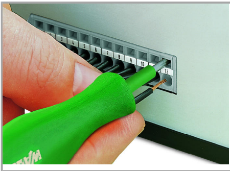
Feedthrough PCB terminal strips – front-entry conductor termination
