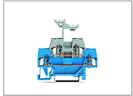
Double-deck terminal blocks accommodate two circuits of different potentials on two decks; different circuits can be differentiated by color coding either deck (280 Series). The lower deck is wider than the upper for ease of wiring.
