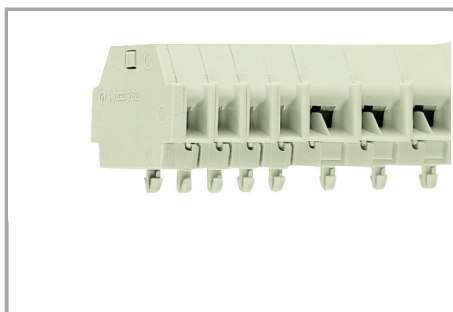
Terminal strip with snap-in mounting feet, for 0.6 ... 1.2 mm plate thickness, 3.5 mm mounting hole diameter (also for 210-154 Aluminum Rail or with 209-120 Mounting Foot for DIN-35 rail)
