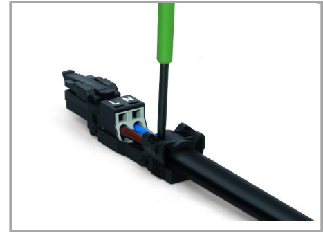
Push down strain relief clamp via 2.5 mm screwdriver alternately on both sides.
