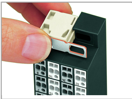
Snapping on an additional module with contact to mounting frame.
