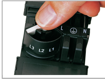
Push down jumper in its new position (picture shows L3).
