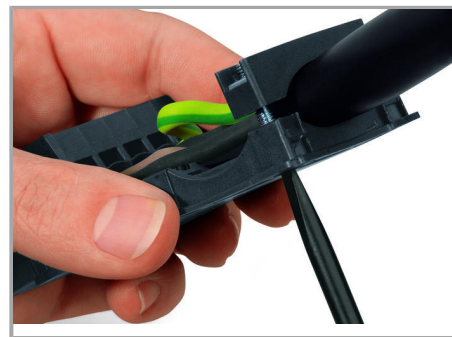
Tighten strain relief using a screwdriver.
