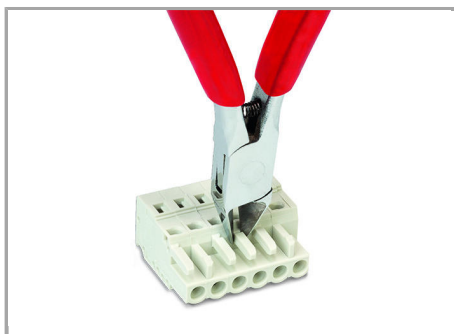
Coding a female connector – removing coding finger(s).
