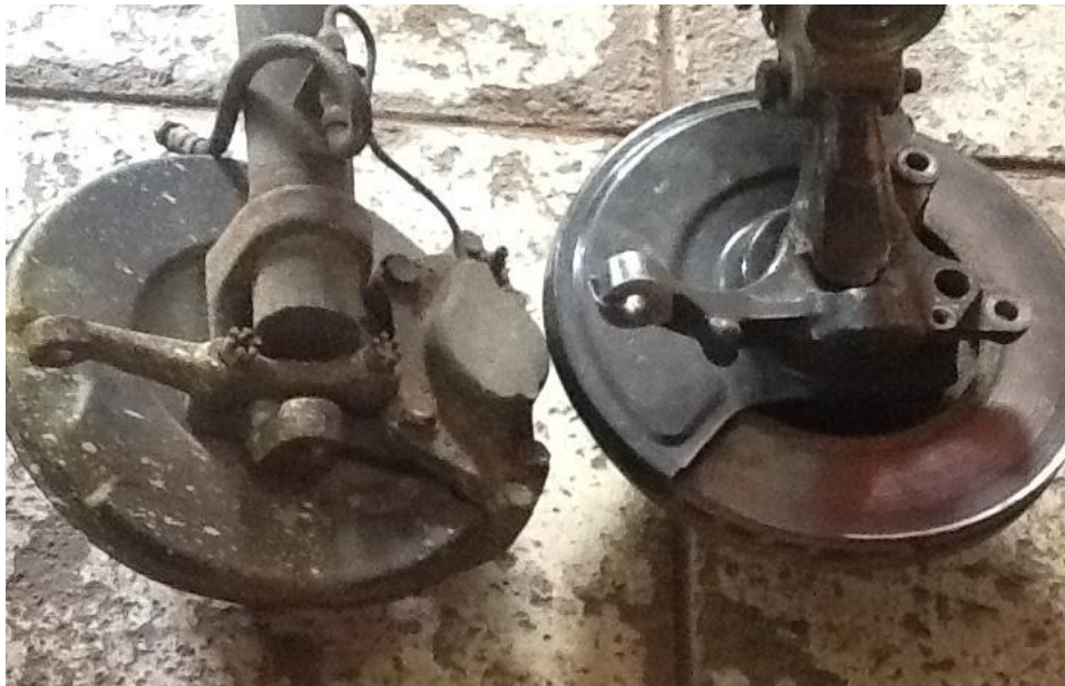
Image above - Ford Capri original strut (left) with Nissan upright (right)
