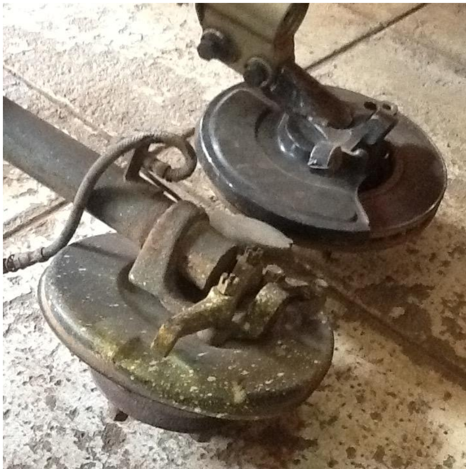
Image above - Ford Capri original strut (left) with Nissan upright (right)
