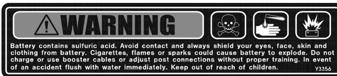
Decal Y3356 – Qty(1) - Place underneath seat plate next to battery compartment.
