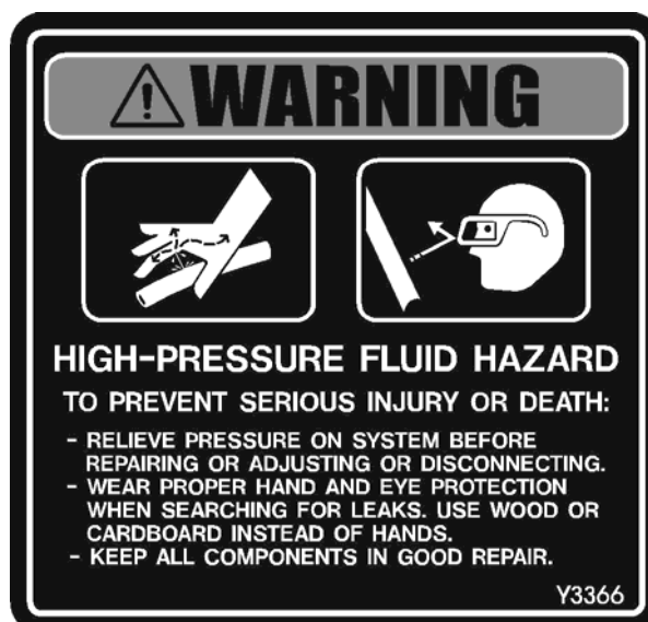
Decal Y3366 – Qty(1) – Place on inside of LH fender, next to seat.
