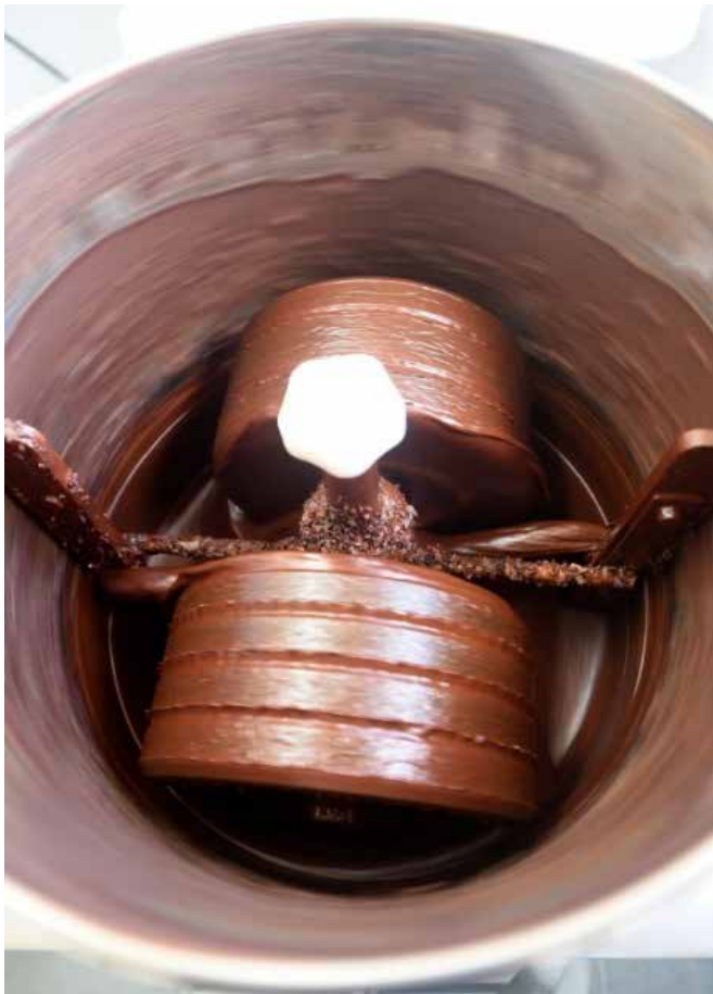
Conche that grinds cocoa nibs to below 20 micron
