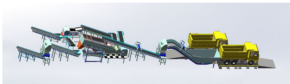
Picture 3: Schematic of recycling equipment of the proposed 10 TPD pilot plant in the Philippines
