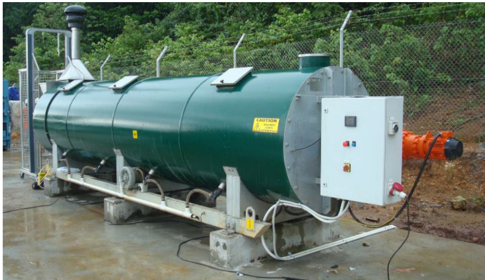
5: Hot Rot In-Vessel Thermophilic Composter (Made in New Zealand)
