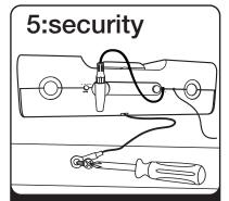
Attach security tether to bottom of the HiH66 and secure the other end to a wall or other permanent surface.
