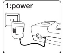
Attach AC adaptor cable to jack on back of the HiH66 and plug the other end into a wall socket.
