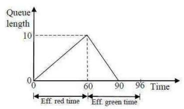
At time t = 0, the light has just turned red. The effective green time is 36 seconds, during which vehicles discharge at the saturation flow rate, s (in vph). Vehicles arrive at a uniform rate, v (in vph), throughout the cycle. Which one of the following statements is TRUE?
