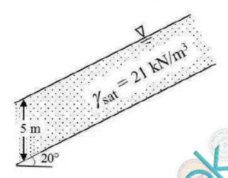
The value of the effective angle of internal friction (in degrees, up to one decimal place) of the sand
