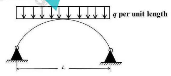
The maximum bending moment in the arch is equal to
