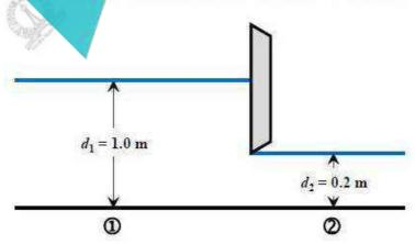
It is observed that the depth of flow is 1.0 m upstream of the gate, while the depth is 0.2 m downstream of the gate. Assuming a smooth flow transition across the sluice gate, i.e., without any energy loss, and the acceleration due to gravity as 10 m/s<sup>2</sup>, the discharge (in m<sup>3</sup>/s, up to two decimal places) passing under the sluice gate is
