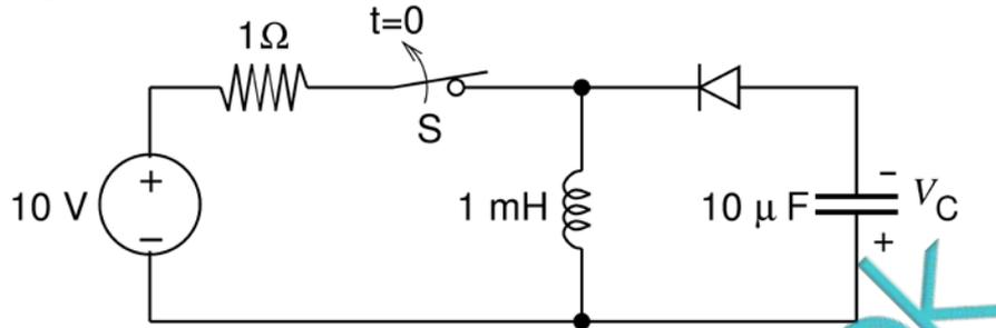
The steady state magnitude of the capacitor voltage  $V_C$  (in volts) is \_\_\_\_\_
