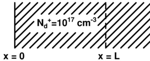
Given  $q = 1.6 \times 10^{-19}$  coulomb,  $\epsilon_0 = 8.85 \times 10^{-14}$  F/cm,  $\epsilon_r = 11.7$  for silicon, the value of  $L$  in nm is \_\_\_\_\_
