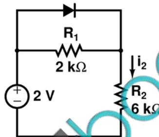
The magnitude of the current  $i_2$  (in mA) is equal to \_\_\_\_\_
