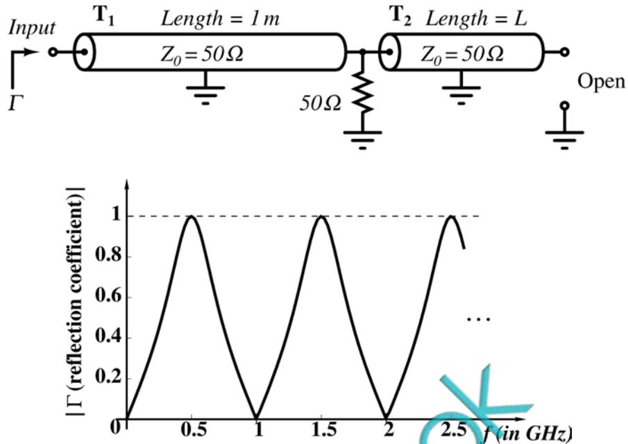
The length  $L$  (in meters) of  $T_2$  is \_\_\_\_\_
