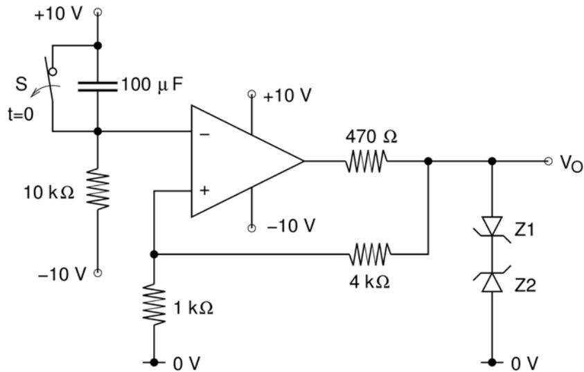
The time  $t = t_1$  (in seconds) at which  $V_O$  changes state is \_\_\_\_\_
