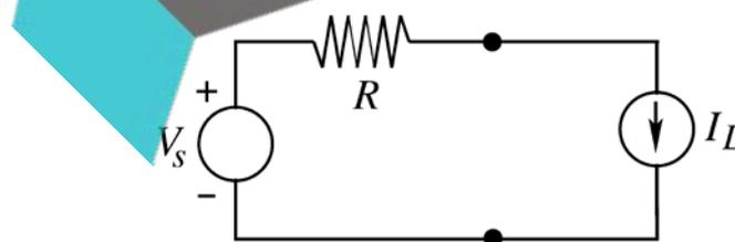
The value of  $I_L$  that maximizes the power absorbed by the constant current load is
