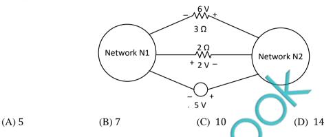
Q.19 For the given circuit, the Thevenin equivalent is to be determined. The Thevenin voltage,  $V_{\text{Th}}$  (in Volt), seen from terminal AB is \_\_\_\_\_
