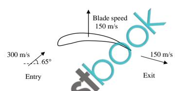
The magnitude of absolute velocity at entry is 300 m/s at an angle of 65° to the axial direction, while the magnitude of the absolute velocity at exit is 150 m/s. The exit velocity vector has a component in the downward direction. Given that the axial (horizontal) velocity is the same at entry and exit, the specific work (in kJ/kg) is
