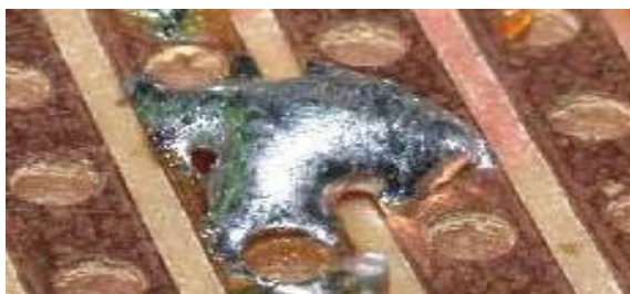
Excess solder on joints
