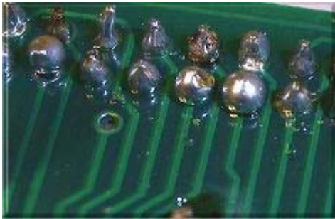
Poor solder joints
