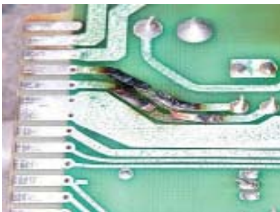
Shows the damage track on PCB
