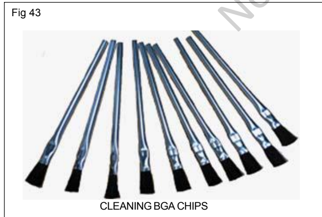
Applicator brushes ( acid brushes) are essential tools in labs and at the bench for cleaning and scrubbing away flux from the circuit board with solvents to remove flux, especially with plated through - hole chips. as shown in fig. 42,43,44,45 &46.
