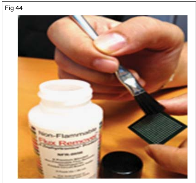
Acid brushes, scrub brushes for PC board repair & rework through- hole, plated through cleaner brushes, flux brushes. as shown in fig. 41.
