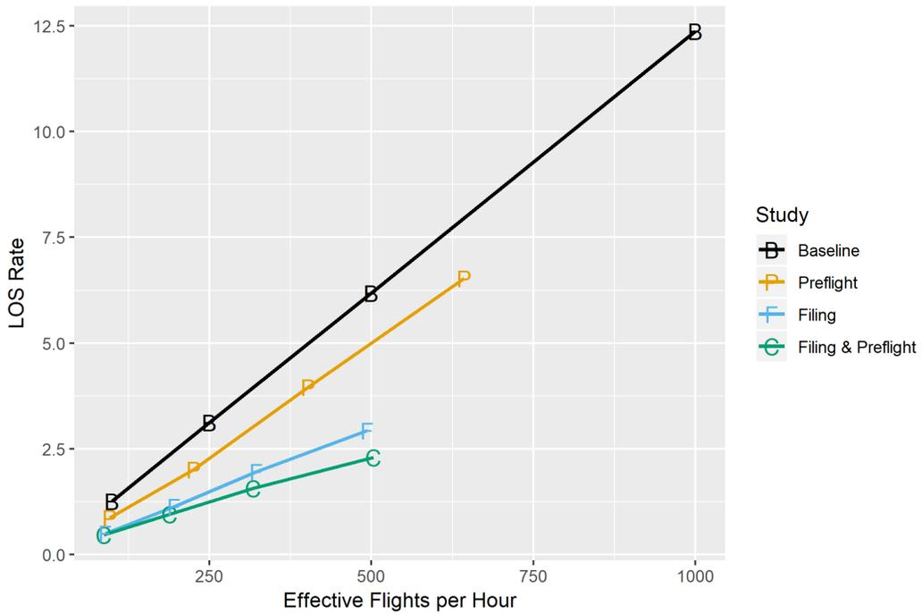
Figure 8: Gaussian Region Loss of Separation Rates
