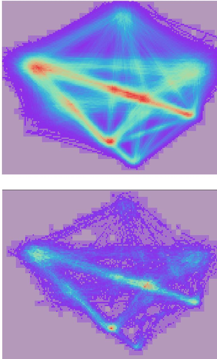
Figure 3: The Shenzhen region at 1,000 flights per hour. The plot at top shows where the most flights operated (orange and red regions), while the plot at bottom shows where the most loss of separation events occurred (green and orange regions) when no preflight airspace management tools were applied.
