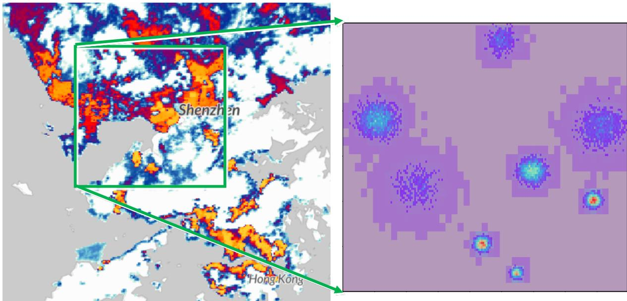
Figure 2: The population density map at left was used to construct the simplified airspace region at right. In the simulated airspace, the most takeoffs occur in the red areas, and least occur in the purple areas. (Source: luminocity3d.org)
