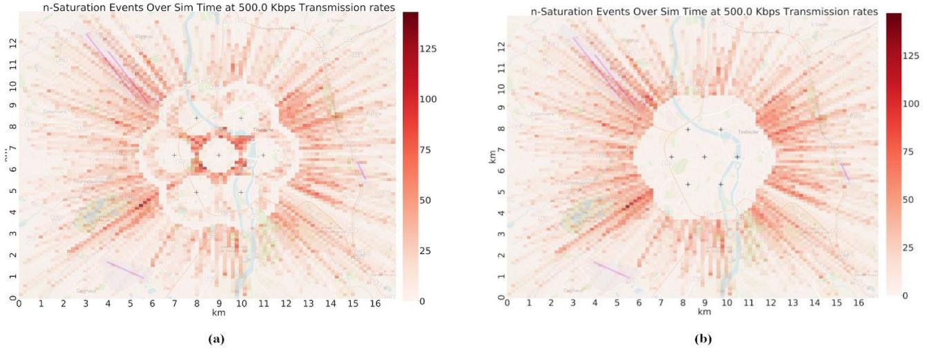
Figure 7. WiFi Cluster Case Study, 500 kbps, high vehicle EIRP, high gain ground antennas, (a) 2 km center-to-center, and (b) 1.5 km center-to-center
