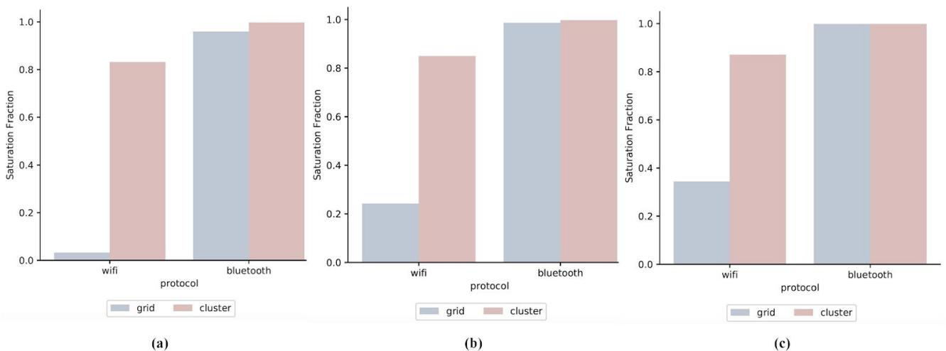
Figure 6. Fraction of saturated vehicles vs configuration for 500 kbps message payload at (a) 250 flights/hr (b) 500 flights/hr (c) and 1000 flights/hr.
