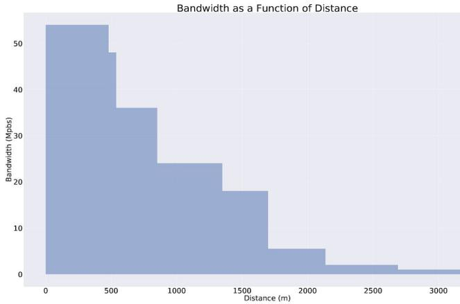
**Figure 3. Bandwidth as a function of distance**
