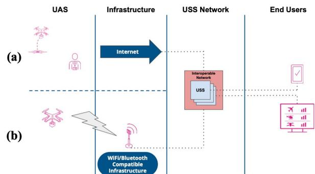
**Figure 1: Remote Identification architecture, (a) Networked, and (b) Broadcast**
