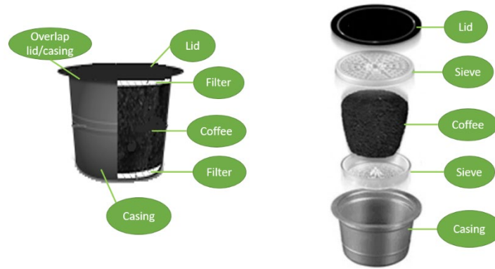
Figure C.1. Examples of typical coffee pod structures
