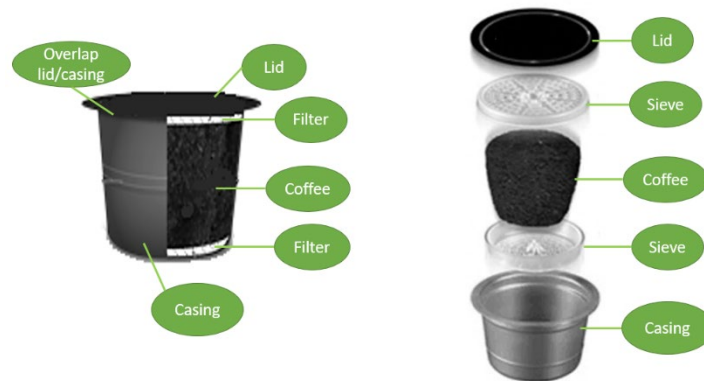
Figure C.1. Examples of typical coffee pod structures
