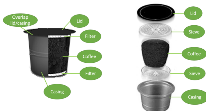
Figure C.1. Examples of typical coffee pod structures
